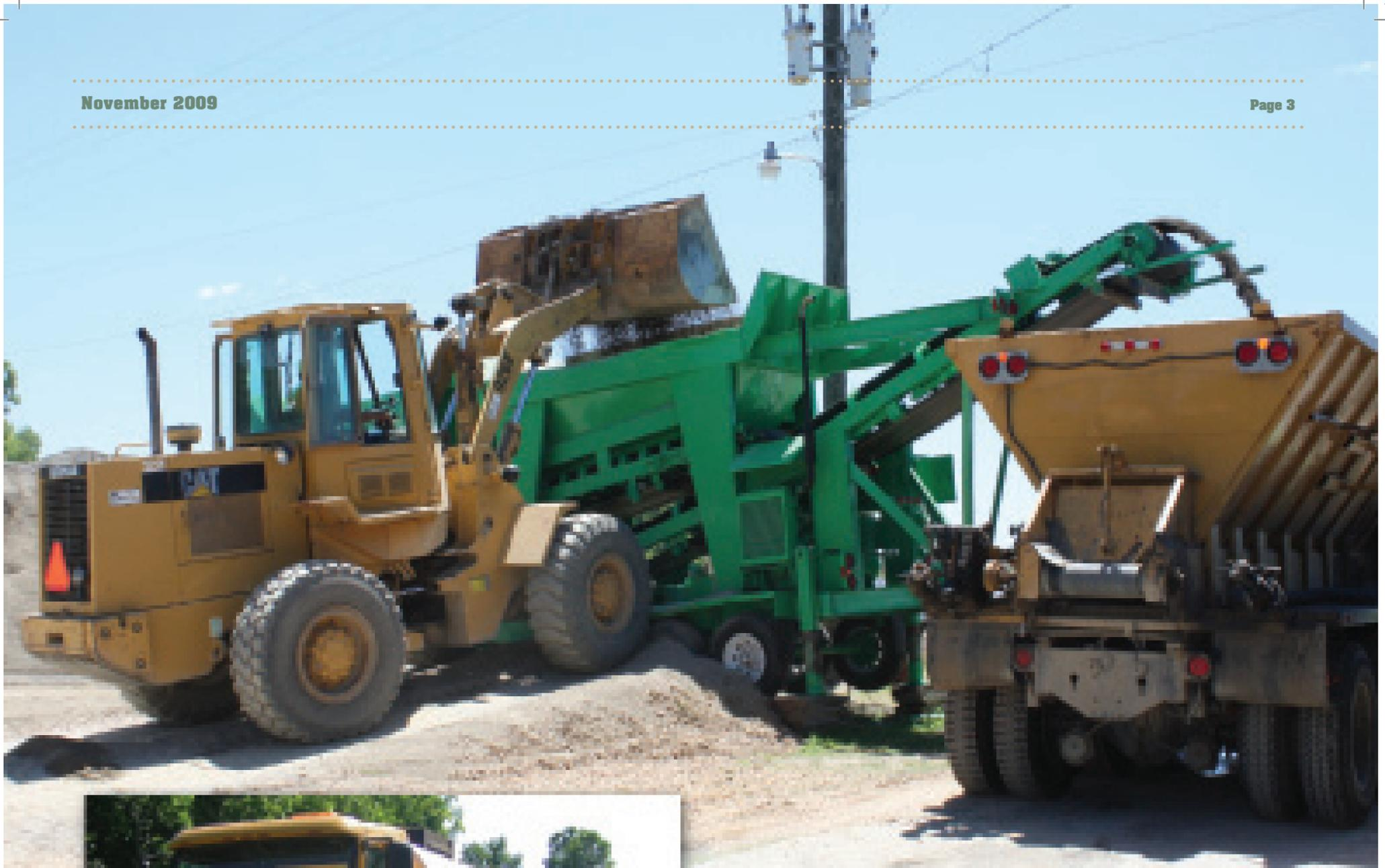
*A CAT 926E loads sandstone into a Rawson mobile plant that screens, weighs and deposits aggregate into a nurse truck.*
